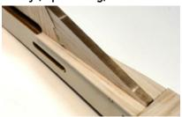
vertical fin. These strips should extend back to the cutout for the horizontal stab, as shown on the plans.
