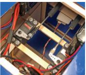
Finish the installation of your radio gear by adding the receiver, flight pack battery and the switch. We mounted the receiver to the fuselage side using a bit of self-adhesive hook-and-loop (not included).
