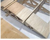
Working on one section at a time, and note that the center gap (between the main spar and the rear sub-spar) will require a couple 1/16th pieces to be edge joined together to cover the gap.
