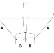
the top fuselage slot, into the stab opening (this might require a bit of sanding on the fin for easy sliding). Once the fin is properly seated, measure the angle between the fin and stab. If at 90°, then it's correct. If not, reposition as needed.
