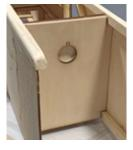
sanding to fit, glue it to the front of F2 to complete the thickened firewall. Use epoxy for this step and be sure to firmly clamp this piece in position while the glue cures.
