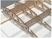
WB3 in place. When satisfied with the fit and location, glue these in place. Working your way inward, attach the other R7, WF3 and WB3 pieces in place.
