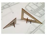
We recommend using the smaller triangle in the wing construction as it's small enough to fit between the ribs.
