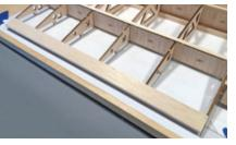
end of each of these ribs. If properly positioned it will also be angled to match the curve of the wing's top surface. When satisfied with the position, glue it in place, making sure it is glued to each of the ribs.
