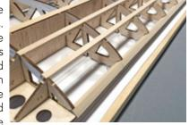
leading edge. Measure, cut and glue this in position. Be sure all three of these strips are glued to each rib.
