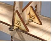
then glue the SS1s in position as shown in the photo. Make sure that one of the SS1s is flush with the bottom of the wing's surface. Once these are in position, mix up a little epoxy and flood the area between the two SS1s to lock the strap in position.
