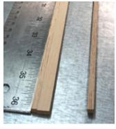
Take one 3/16" x 3/8" basswood piece and lay it on your board. Glue one of the 3/16" balsa sticks to each side of the basswood as shown here to make one strut assembly.
