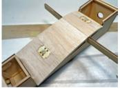
Use caution to make sure the wing does not move until both holes are drilled.
