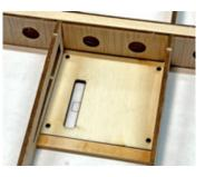
place on the plans, between the ribs and up against the lower spar. Now SW3 will be installed to form the 4th side of the aileron box. It should be snug up against both ribs, and loosely against SH1. I say loosely because you'll want to leave a touch of room to account for the thickness of covering to be applied later.
