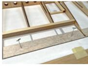
side of the R6 ribs. Pin this in position.
