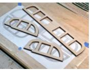
remove these assemblies and flip them over and lightly sand the framework. Then glue the other set of ST13/ST12 to the assemblies.
