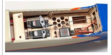
Take a bit of time to plan things out, including how you'll run the throttle and nose gear steering pushrods.
