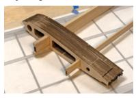
same direction. Double, triple, and quadruple check that you have them in the correct order, then when satisfied, push the front spar into the larger rectangular hole in each rib. The rear spar is pushed through the smaller rectangular hole towards the rear of the ribs.
