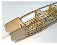
When satisfied with this dry fit, remove the tray, apply glue, and put in back in position. Make sure it's held in place and that the fuselage sides continue their gentle curvature that is cut into TR2.
