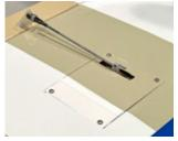
Finish the layout of your radio gear by adding the receiver, flight pack battery and the switch. We mounted the receiver to the tray by using a bit of self-adhesive hook-and-loop (not included). The radio's switch should be mounted to the opposite side of the muffler (to help keep the goop out of it). Or, for an even cleaner installation, it could be installed inside the tank/battery compartment - hidden under the hatch - VERY NICE!
