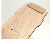
Now test fit BS1 in place on top of the fuselage, and note how it fits into the tab on F6, as well as resting on the bottom of F4. The side tabs will fit into the notches cut into the fuselage sides and should be flush with the sides when installed correctly.
