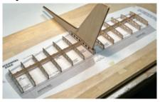
one side of the stab, then the other. Take the time to make sure everything is aligned properly BEFORE you glue it in place, as it's just about impossible to fix if things are out of order and glued in place. When finished, you should have something that looks just about like this photo.
