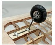
landing gear straps as shown in the photo. Use a 1/16" drill to make the mounting holes for the screws, and then attach the straps in position.
