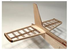
Now, if you take a measurement from the flat of the building board to tips of the trailing edges, they should be the same distance (giving you a nice, horizontal stab). If adjustment is needed, lightly sand the taller fuselage side to lower the higher side.
