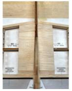
especially against the tapered edge of the leading edge. What you want is a piece that fit snugly against the leading and trailing edges as shown here.
