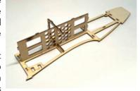
together, apply glue to the edges of the TR1 assembly, everywhere it will contact FSP. Glue these two pieces together, making sure that the tabs are fully inserted in each of FSP's slots.
