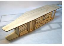
Take one of the balsa sides from the previous step and you will now glue it to one of the sides of the plywood assembly. Be careful to line it up exactly and make sure it stays in place as the glue cures.
