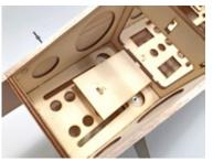
to mount you batteries. The idea is to raise up the tray level with T2, so larger and longer batteries can be used. Also it allows the batteries to be shifted aft if needed, for C.G. purposes.
