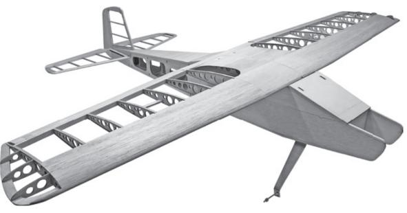
**Specifications**: Wingspan: 60 in. • Wing Area: 710 sq in. Airframe Length: 49 in. • Weight: 4.5 - 6 lbs. (ready to fly)
