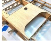
The design of the wing will also make this sheeting flush with trailing edge.
