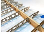
the ribs. These strips will need to bend slightly around R4, so make sure to keep pressure (or weight) on them until the glue has cured.
