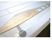
join so you end up with a smooth side. When finished, repeat this step to make the other balsa fuselage side.
