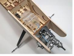
mounting it as shown here on one of our Javelin prototypes. This particular engine required an muffler extension to space the muffler away from interfering with the bottom of the fuselage.
