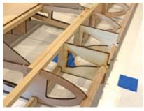
tune the positioning of the R1E or R1G pieces over the plans. Make sure they are 90° to the building board and that they're seated on both the upper and lower spars.
