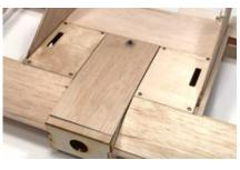
When in place, use a 1/16" bit to drill through the 4 pre-cut mounting holes in each hatch, into the 1/4" basswood underneath. Later on, you can use the supplied  $2-56 \times 3/4$ " self tapping screws to hold these in position.
