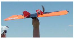
to what's shown here - by the skid, throttle up, then throw the Bat forward and just slightly nose-up. **And I do mean slightly - not 45°.**
