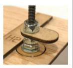
allow the bolt to turn in the hatch freely, and without a lot a slop. Now thread on one of the 4-40 lock nuts all the way to jam against the 4-40 nut previously installed.
