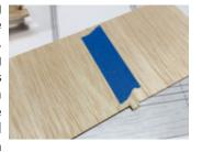
hinge allowing you to put a small amount of adhesive in the joint. When the adhesive is applied, place the sheeting back down on the waxed paper, so that it's flat (as shown in the photo). When cured, you'll now have a single, longer piece of sheeting.
