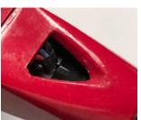
you make a "cheater hole" in the bottom of the cowl, similar to this, so cooling air can enter the fuselage.
