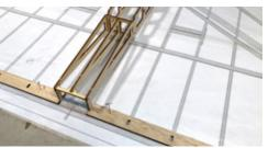
as shown on the plans, over the trailing edge. Use a long straight edge to assure that both edges line up. The inner notch will fit around the extended tab on the back of the R1 pieces.
