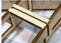
We recommend dry-fitting these first, then gluing together. Try to keep glue out of the slot in G1 as this is where the main landing gear will be mounted.
