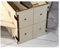
the mounting holes. Lightly tap the blind nuts into place on the back of the firewall and secure them with a bit of glue. When finished, skip to step 43.
