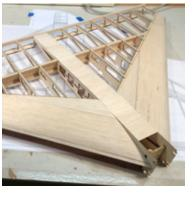
Work from the rear of the center section, forward. You'll need to cut and join a few pieces together but be sure to stop an inch or two behind the F5 (nose gear mount). You'll need this open to aid in mounting your powerplant.
