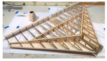
Once all the glue has cured, remove the Comet assembly from the building surface and flip it over.
