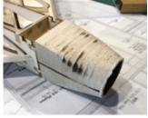
Now, to hold the cowl in position, drill into the holes in each cowl mounting tab using a 1/16" bit. Make the holes about a 1/2" deep. Using 4 of the supplied 2-56 x 3/4" self tapping screws, attach the cowl to the Comet.
