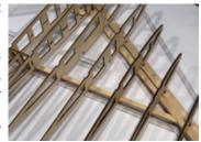
When satisfied with the alignment, glue the front and rear spars in place, making sure they are attached to all of the ribs and to each other.
