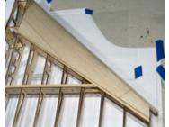
each of the ribs. As a general rule, don't use super-fast curing C/A's for the step as you will need a bit of time to make sure everything is in place.
